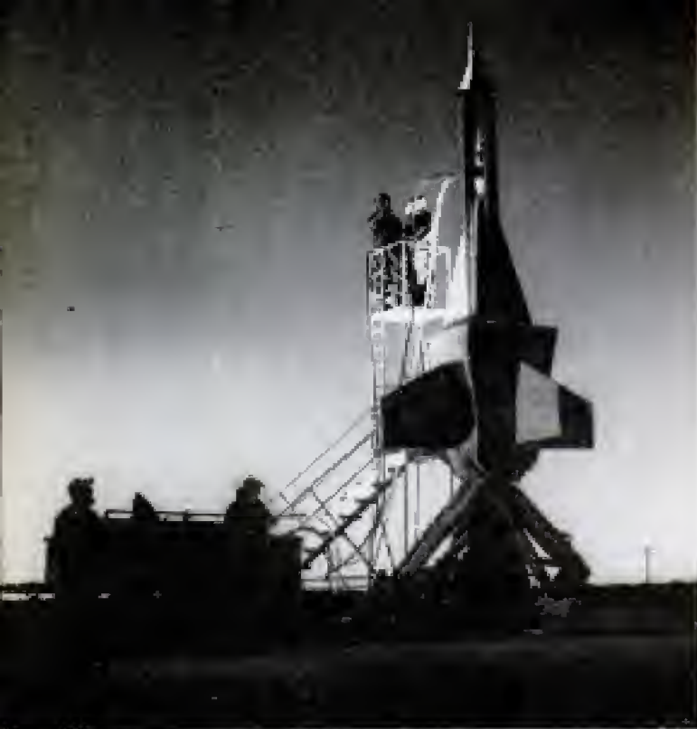
Being fueled for a dawn launching, the Nike missile is handled by men (at top) wearing antacid gear
